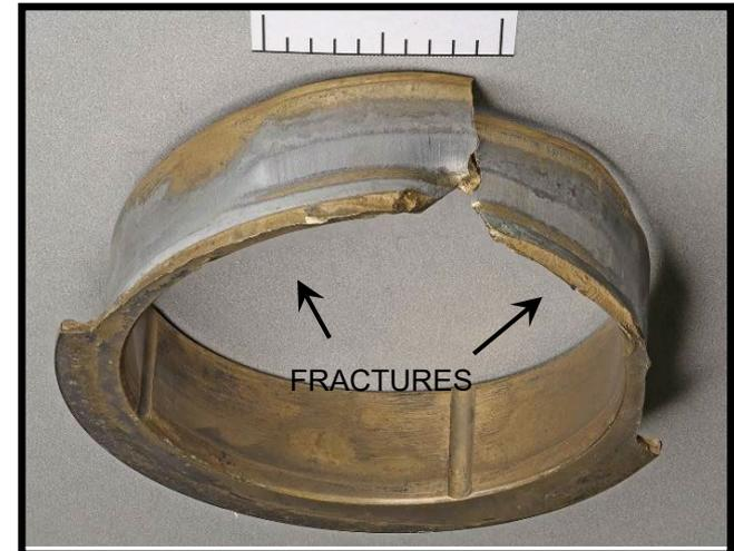
Figure 97. View of MLG- Universal Side Strut FWD Bushing.
