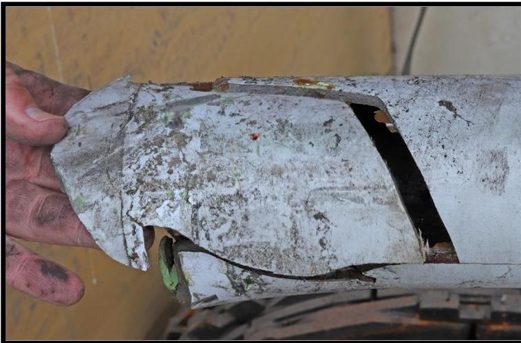
Figure 45. Detailed view of Upper Drag Strut- Fracture.
