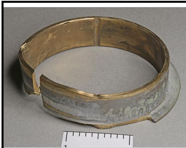
Figure 96. View of MLG- Universal Side Strut FWD Bushing.
