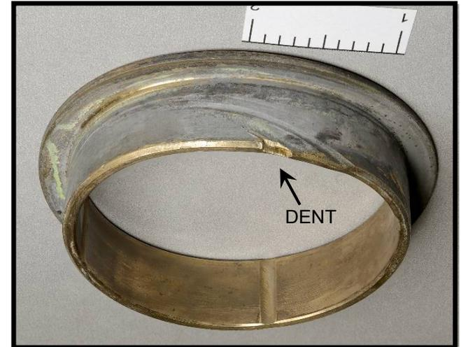
Figure 95. View of MLG- Universal Side Strut AFT Bushing.
